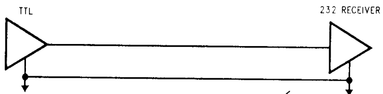
FIGURE 8. TTL to RS-232
